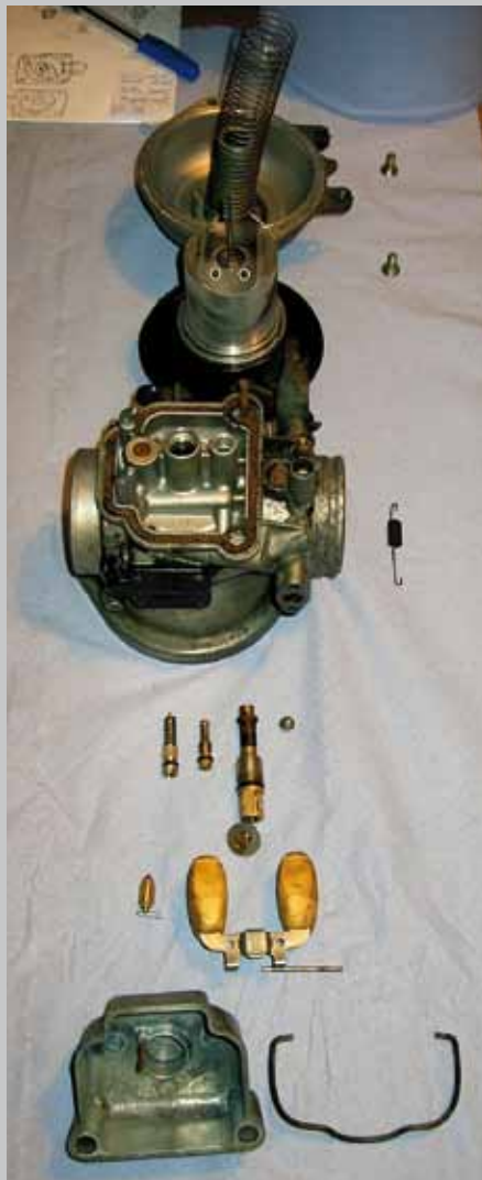
To get to the MoT I needed the bike to run properly. This was largely achieved by rebuilding each carburettor
