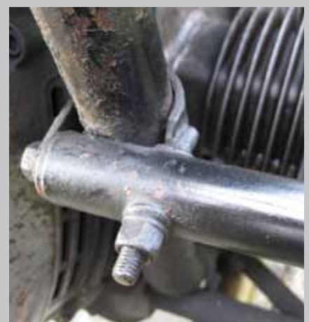
The bolts (or maybe they're studs?) on the right-hand engine bar clamps sheared when I tried to undo them. This clamp's on the left-hand bar and the threads look OK. I'll leave it be for now though!
