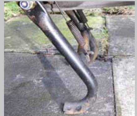
The curved tubes allow a smooth lift up onto the centrestand. Unless they have rusted through and had chunky patches welded on...
