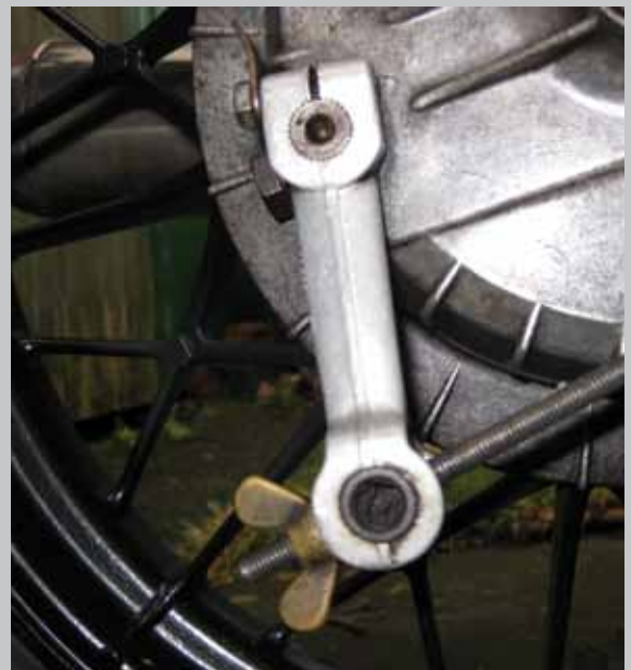
Replacement for the broken cam lever. It's secondhand but shows none of the original's corrosion
