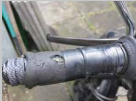
Heated grips had been fitted, but the covering had worn through to the element and they didn't work. For a slightly neater finish I wrapped insulating tape around them, running out before quite finishing the left one
