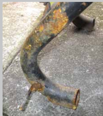
This is the bit of metal rod I welded on as a tang. The picture also demonstrates that one thick coat of paint is not as good as two light ones
