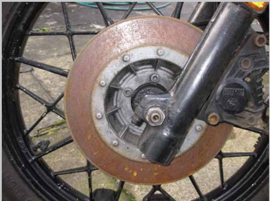
Horrid looking iron disks have been fitted that shed a lot of rust. In case this was somehow causing the brakes to bind I cleaned off the dust round the pistons and pads
